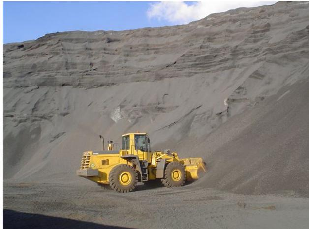
According to [the SOLAS 1974 Convention](#), the shippers are obliged to provide valid certificates declaring the moisture content as well as the transportable moisture limit (TML) of any type of cargo being able to liquefy. It is imperative that these two figures are identified at the time of loading, especially if the cargo is known to have been left out in the open prior to loading. The moisture content should not exceed the TML. Otherwise the result may be liquefaction and shifting of cargo.
