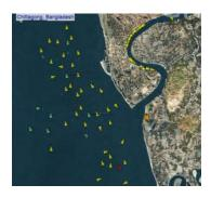
With the Patenga light beacon bearing more than 055°, the seabed is soft mud and vessels are liable to drag anchor. With the Patenga light beacon bearing less than 055°, the holding ground is relatively firm but attention must be paid to the strength of the ebb tide<sup>1</sup>, especially during the monsoon months (normally June to November).
