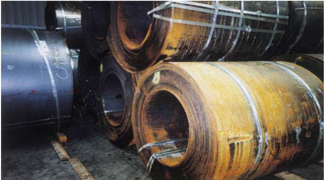
Condensation damage to steel coils.
