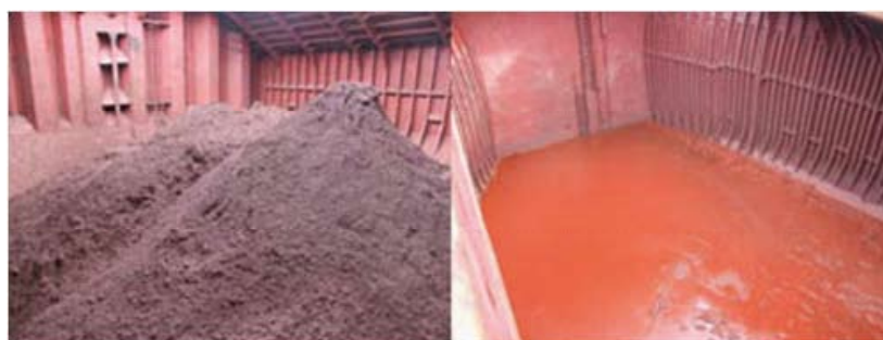
Iron ore fines before and after liquefaction.
