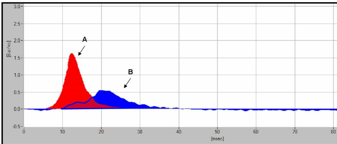
**A:** Reference curve. Normal peak pressure and an ignition delay of 5.9 ms (millisecond). Start of main combustion, 7.85 ms.
